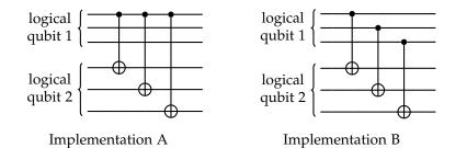
(5) Assume that the only sources of errors are individual controlled-NOT gates which produce bit-flip errors in their outputs. These errors are independent and occur with a small probability *p*. For each of the two implementations find the probability of generating unrecoverable errors at the output. Which of the two implementations is fault-tolerant?
